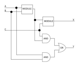
There is another circuit board called MODULE, which produces R from P and Q:
